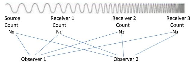
The observers see the streaming of wavefront counts data No N1 N2 and N3 are all synchronized with constant differences. This is true as long as the receivers and observers are stationary relative to each other.
